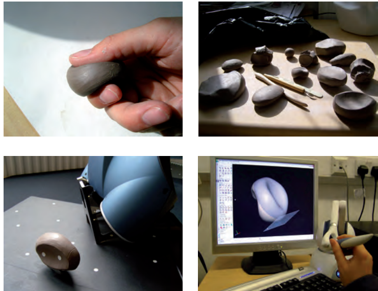
Figure 1, Using advanced tools (i) form by hand (ii) using conventional tools (iii) digitally scan (iv) use Phantom arm haptics to edit digitised solid
