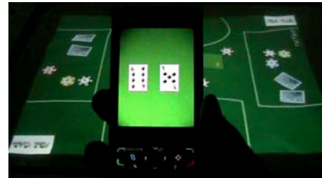
Figure 1: Poker Surface: an example application integrating mobile phone interaction and a multi-touch table.
