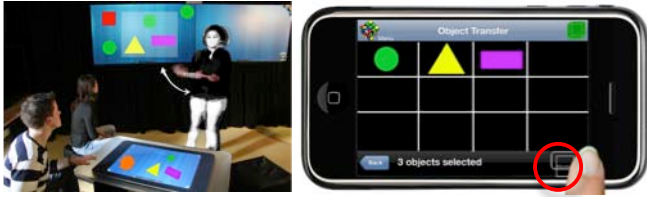
Figure 2. User turns to the target display. She transfers the selected objects to the target display by tapping on the icon of that display (the icon under the red circle).
