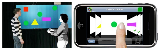
Figure 1. User selects her objects of interest using an iPhone. iPhone shows the selected objects, as well as the current display in focus.
