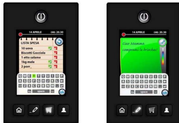
Figure 5 A and B On the left the user interface to add items to the shopping list, that may be updated also by the ZmartFRI. On the right the user interface to write a message for an house resident.
