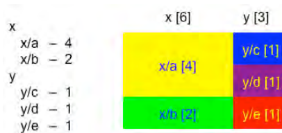
Fig. 16. TreeMap of two level hierarchical data: data on the left, TreeMap on the right
