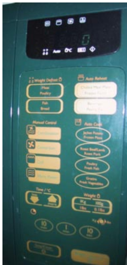
Figure 5.9 Microwave control panel
